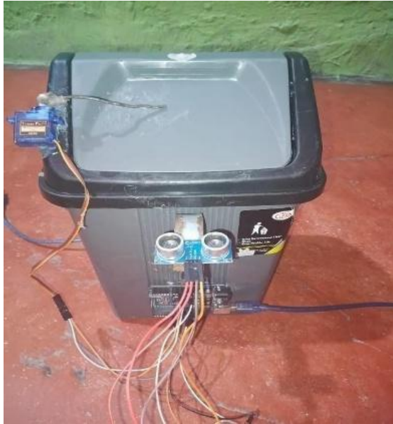
Figure 2. Trash Bin Prototype Tested with Arduino
