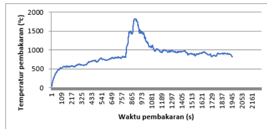
Figure 7 Graph of combustion temperature of organic waste charcoal particle pellets, mixture (1; 5; 10%).
