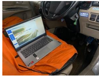
Gambar 2 Scanner Mongoose ( Socket DLC OBD II )
