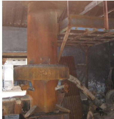
Figure 3 Single tuyere cupola furnace in Ceper. (Photograph taken by the author during fieldwork).
