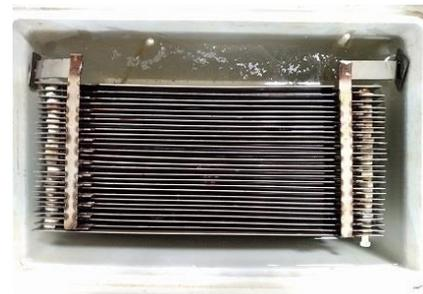
**Figure 3** Stainless Steel Electrode
