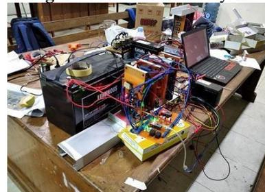
**Figure 5** Buck Converter and Datalogger
