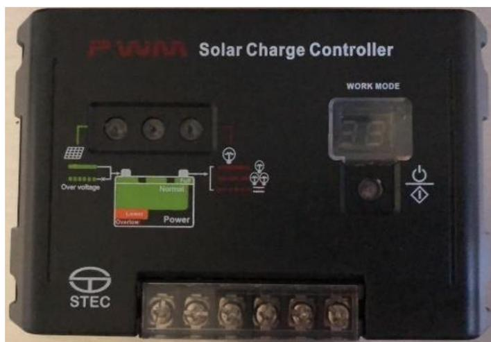
Gambar 15. Board pengendali pengisian PWM Solar charge controler (SCC)
