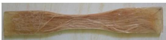
Gambar 1. *Specimen composites* ASTM D-638 type III
