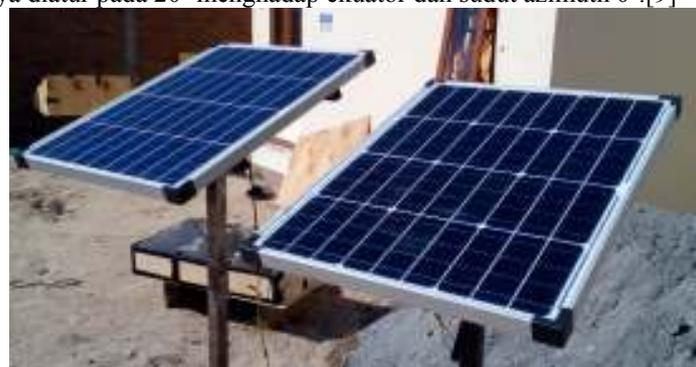
Gambar 2. Set up panel surya *polycrystalline* dan *monocrystalline*
