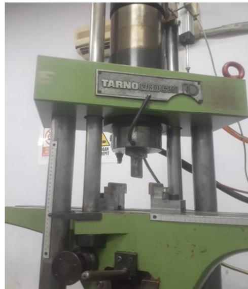
Gambar 2 Uji *three-point bending*
