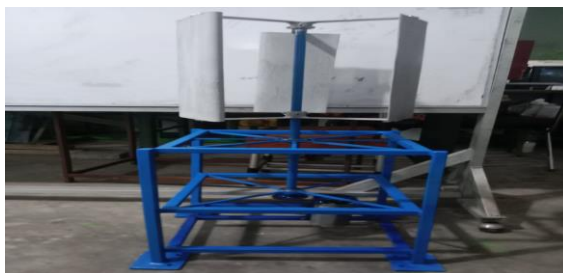
Gambar 1 Wind Turbine Jenis Darrieus Tipe H
