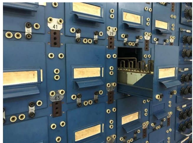
Fig. 3. ITU Power Systems Lab. Analog Energy Transmission Simulator, Pi and T model modules
