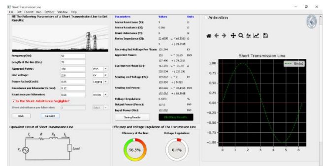
Fig. 7. ITUPSA Short Transmission Parameters and Transmission Line Analysis.
