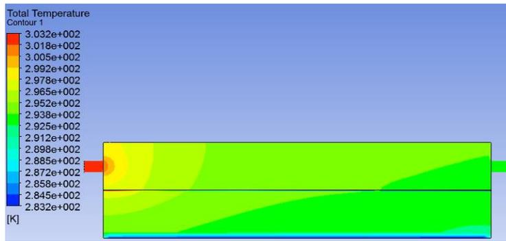
**Figure 3 Visualization of temperature distribution using cylindrical nozzle**
