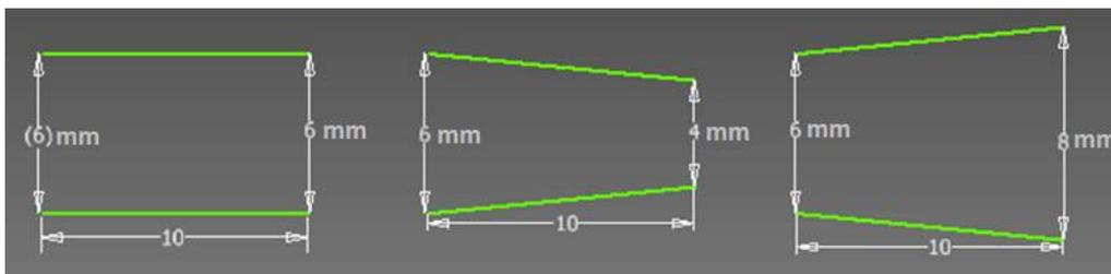
**Figure 2 The cylindrical, convergent and divergent nozzles**
