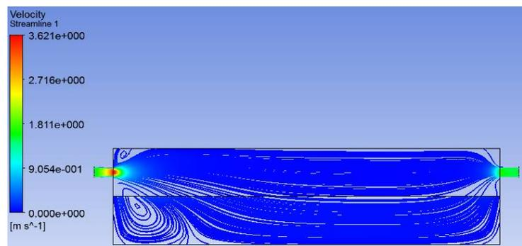
**Figure 7 Visualization of fluid flow using convergent nozzle**
