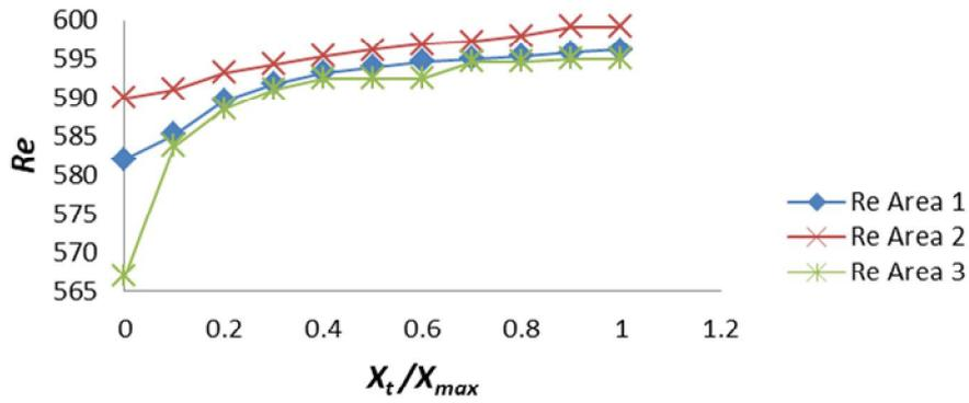
Figure 12 Reynolds number with cylindrical nozzle
