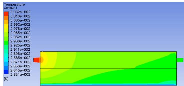
**Figure 5 Visualization of temperature distribution using divergent nozzle**
