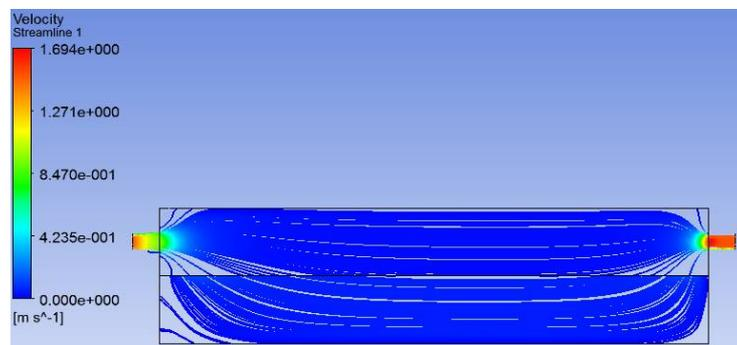
**Figure 8 Visualization of fluid flow using divergent nozzle**
