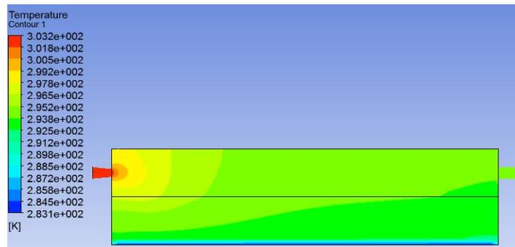
**Figure 4 Visualization of temperature distribution using convergent nozzle**
