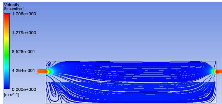
**Figure 6 Visualization of fluid flow using cylindrical nozzle**
