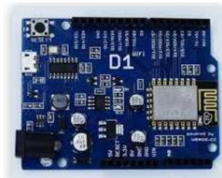
**Gambar 4.** Arduino ESP 6288 D1 wemos wifi
