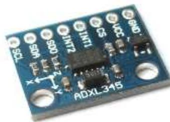
**Gambar 5.** Modul Accelerometer ADXL345 3-axis
