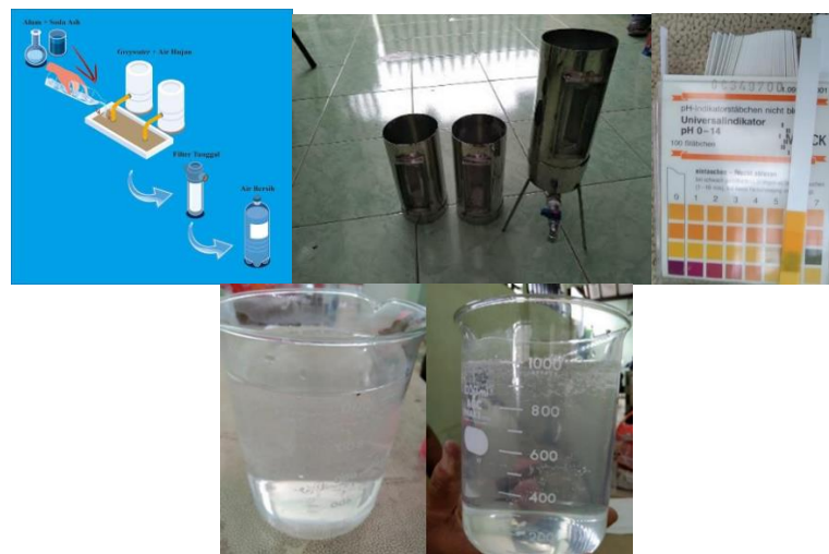
Gambar 4. Gambaran Iptek Proses Filter Air Bersih, Alat test filter, alat pH, air sblm dan air sesudah treatment
