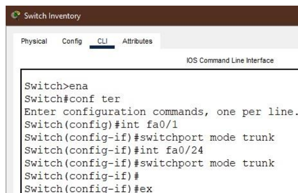
Gambar 13. Switchport inventory mode trunk
