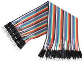
Gambar 4. Kabel Jumper
