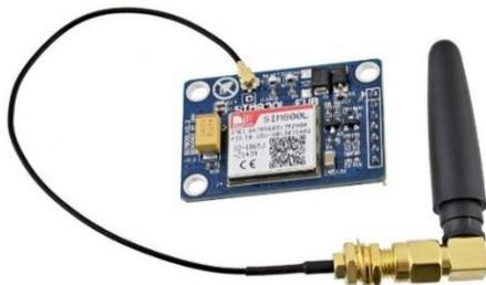
Gambar 2. Modul SIM800L V2
