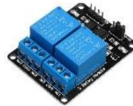
Gambar 3. Module Relay 2 Channel 5V
