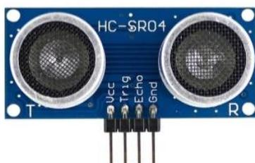
Gambar 2.3 Sensor Ultrasonik
