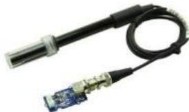
Gambar 4. Sensor ph 4502c
