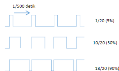
Gambar 18. Duty cycle Sinyal PWM
