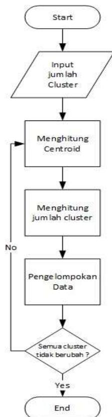
Gambar 1. Flowchart Algoritma *K-Means*
