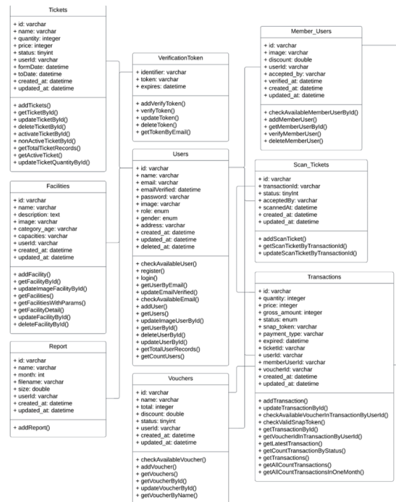
Gambar 3. Class diagram sistem e-ticket
