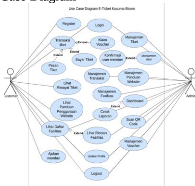
Gambar 2. Use case diagram sistem e-ticket
