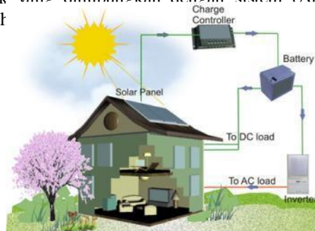
Gambar 1. Sistem Instalasi Panel Surya
