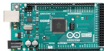
Gambar 1. Arduino Mega 2560
