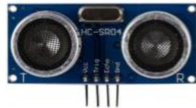
Gambar 2. Sensor jarak ultrasonic
