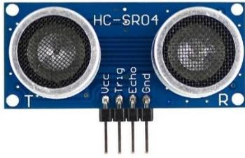
Gambar 9. Sensor Ultrasonic HC-SR04
