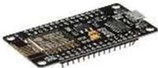
Gambar 1. NodeMCU
