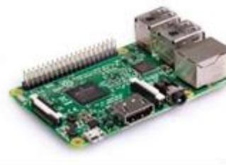
Gambar 2. Raspberry Pi 3 model B+
