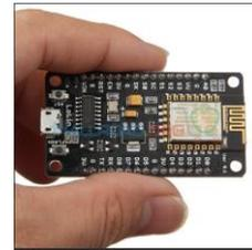
Gambar 9. Nodemcu Lolin V3
