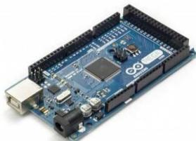
Gambar 2. Arduino Mega
