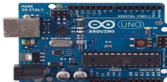
Gambar 2. Arduino Uno Board
