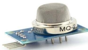
Gambar 3. Sensor Asap MQ-2
