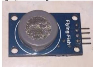
Gambar 4. Sensor Gas MQ-7
