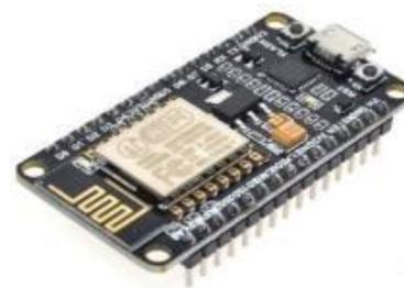
Gambar 1. NodeMcu ESP8266
