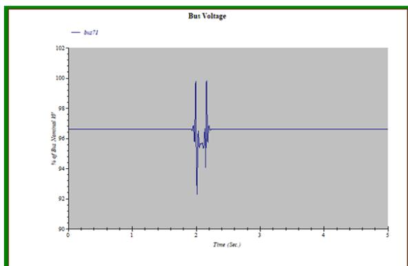
Gambar 3. Busbar 71 Setelah Integrasi PLTS
