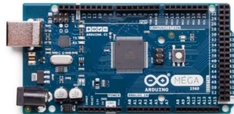
Gambar 5. Arduino Mega 2560
