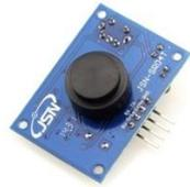
Gambar 4. Sensor Ultrasonic JSN-SR04T
