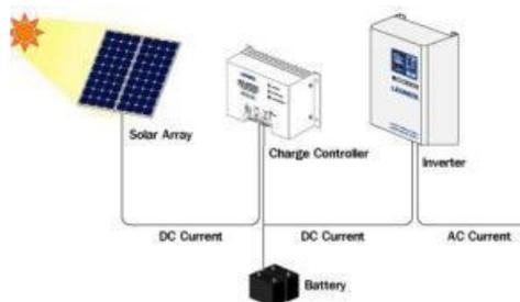
**Gambar 6:** Sistem Energi Surya Fotovoltaik
