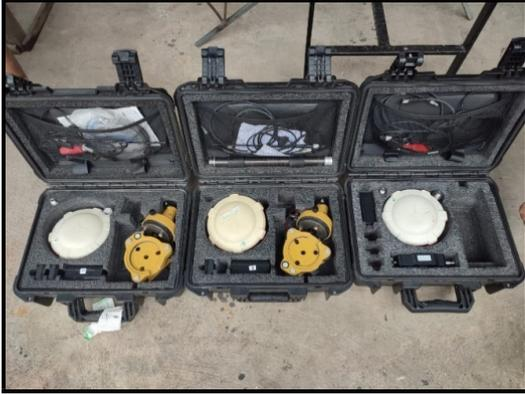
Gambar 2. Peralatan survei receiver GNSS
