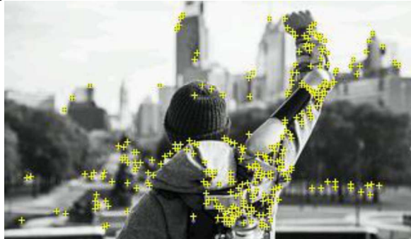
Gambar 5. Proses tracking image target di vuforia
