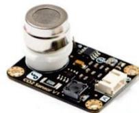
Gambar 2 Sensor MG811<sup>[5]</sup>
