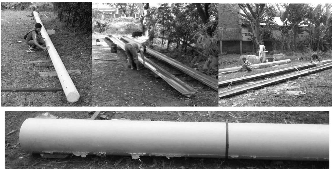
Gambar 6. Proses Pembuatan Tiang Fiberglass Reinforced Composite [6]
