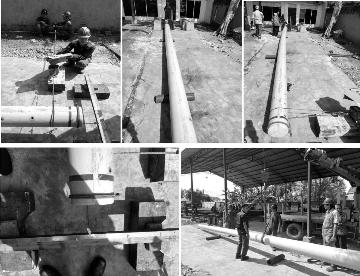
Gambar 7. Proses Pengujian Tiang Fiberglass Reinforced Composite [7]
