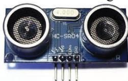
Gambar 7. Sensor Ultrasonik
