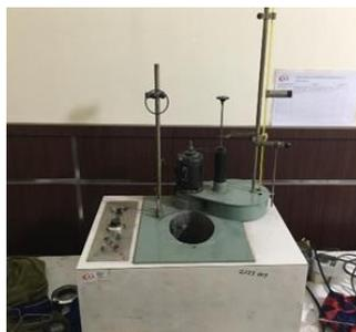
Gambar 2. Bomb Calorimeter
