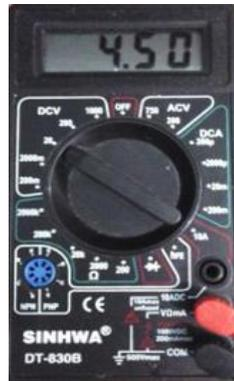
Gambar 3. Output Dari Sensor Tegangan Pada Batere
