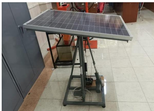
Gambar 6. Solar panel tracking system
