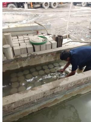
Gambar 7. Proses Curing
