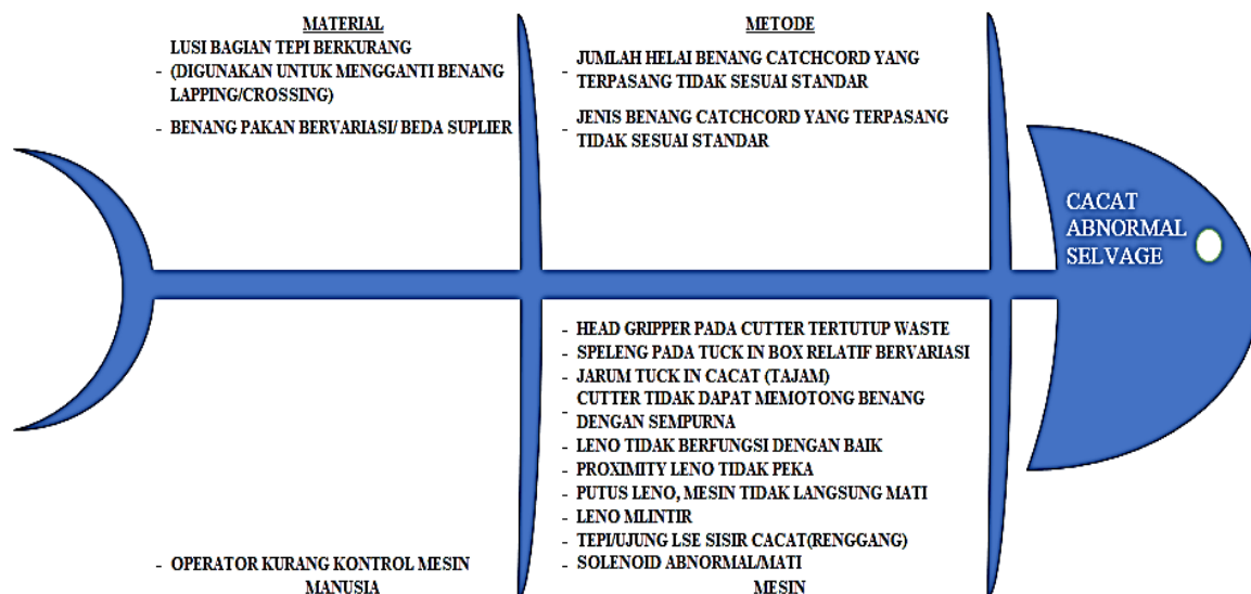
Gambar 2 Diagram fishbone cacat abnormal selvage
