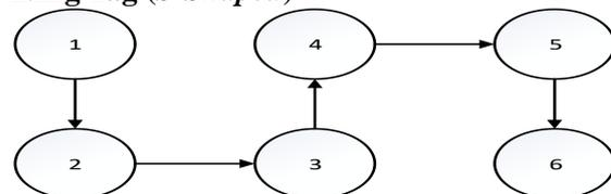
Gambar 2. 2 Pola Aliran Material Zig-zag (S-Shaped)
