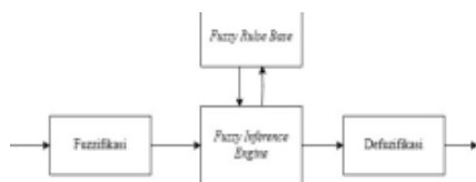
Gambar 4. Tahapan Metode Fuzzy Logic
