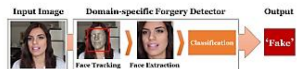
Figure 2. Domain-specific forgery detection pipeline for facial manipulations: the input image is processed through robust face tracking, followed by face extraction, and the cropped region is fed into a classification network that outputs the final prediction (real or fake)
