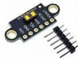
Gambar 3. Sensor jarak berbasis time-of-flight (ToF) VL53L1X ToF
